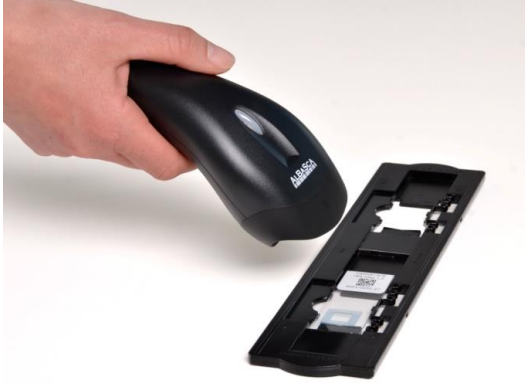
Figure 10: Hand scanner and chip in a slide holder
